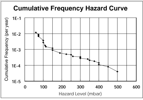
From this curve it can be seen that the design hazard level is just over 400 mbar. This is a significantly different result to that obtained if all events less frequent
